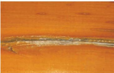
Fissure with peeling.
