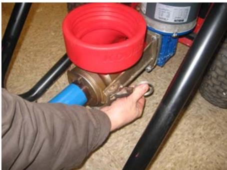
If the rotor is inserted far enough and the connecting drive shaft is aligned, the assembly will connect back into its original position and can be locked back in place. The Rotor-Stator Assembly is complete.
