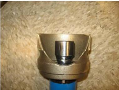
The rotor should stick out approx. 2" as shown above, making sure the gasket in the brass retainer stays in place.
