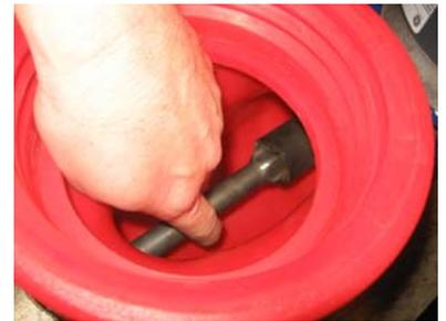
The connecting drive shaft must align with the square receiver on the rigid coupling.
