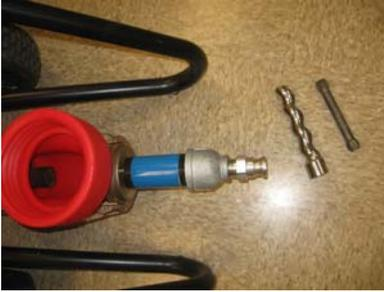
Unwrap rotor and connecting driveshaft.
