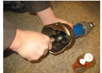
Screw and push the rotor into the stator tube, counter-clockwise.
