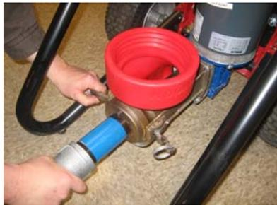
Slide the rotor-stator assembly into the pump housing base. If the assembly does not go all the way back, check the connecting drive shaft alignment.
